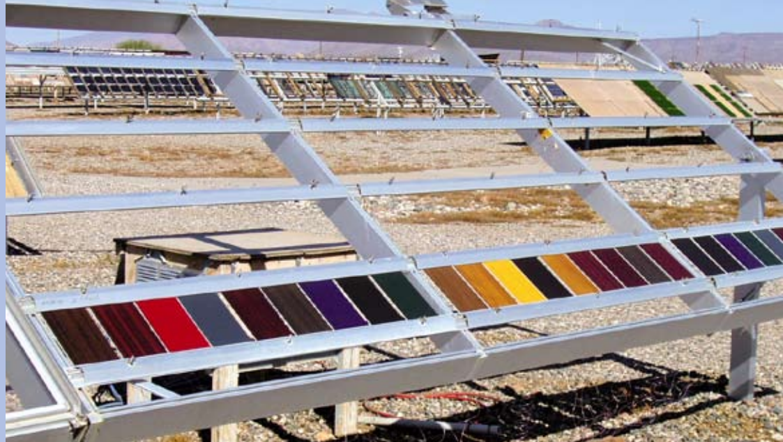
Desert Grill: RENOLIT film with SST in a durability test in the relentless Arizona sun.
