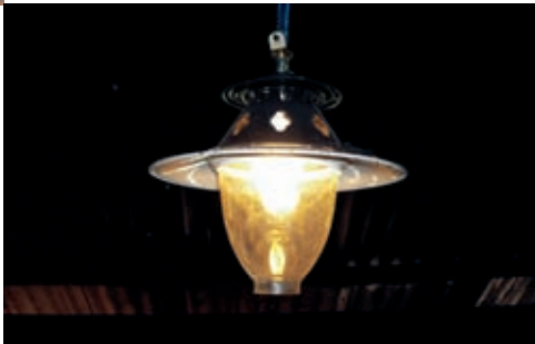
This gas lamp is illuminated with biogas.
